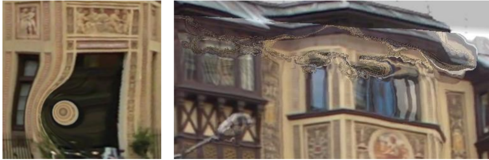
Figure A.7: Artefacts in the warp transitions, taken as zoomed regions of Figure A.6. Left: Swirl artefacts from incorrect feature point correspondence. Here, a feature to the left of the door has been matched with a feature to the right, causing the warp to generate a swirl. Right: Flickering at the boundary between images, where the flow between the two overlaid images is undefined.
