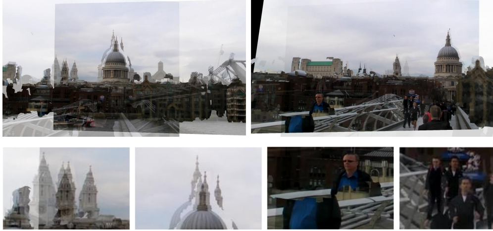
Figure A.14: Top: Two frames from a full 3D dynamic transition which contain artefacts caused by incorrect geometry. Bottom: Zoomed sections highlighting specific issues. From left to right: multiple geometry features (three/four on the tower, then three on the dome) and inaccurate dome geometry with sky recovered as geometry causing a halo effect; split pedestrian, where his head and shoulders are projected onto scene geometry and his torso onto the ground plane; double projection of a runner, again one onto the scene geometry and one onto the ground plane.
