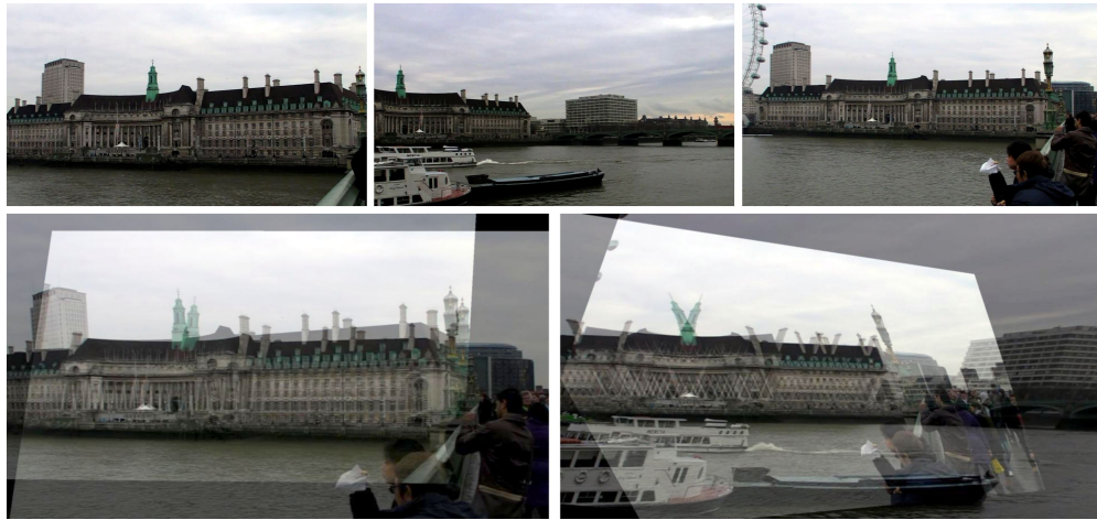
Figure A.8: Top left: Slight view change start frame . Top middle: Considerable view change start frame . Top right: End frame for both transitions . Bottom left: Middle frame of a plane transition for the above slight view change. Ghosting is visible on static objects due to camera translation . Bottom right: Middle frame of a plane transition for the above considerable view change. Ghosting on static objects is visible as before, but the large translation and rotation causes buildings to appear skewed .
