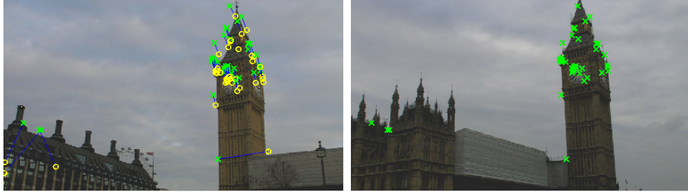
Figure A.3: These two portal frames break the 180^\circ cutting rule, as they are taken from opposite sides of Big Ben. SIFT features have been matched and verified on the tower even though the surrounding buildings are different. Yellow circles in the left frame are matched to green crosses in the right frame. Green crosses in the left frame show the relative offset from the original position of the yellow circle feature point in the left frame.
