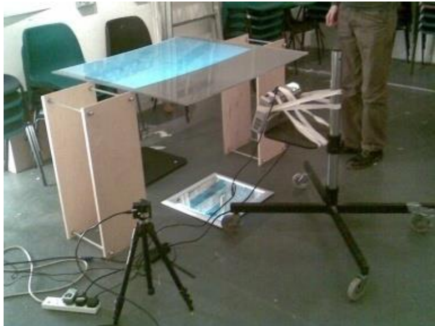
Figure 22: Testing the polycarbonate's suitability for a multi-touch table, bearing in mind the polycarbonate is 10mm thick. Due to the large size of the table, the surface needs to be structurally self-supportive.
