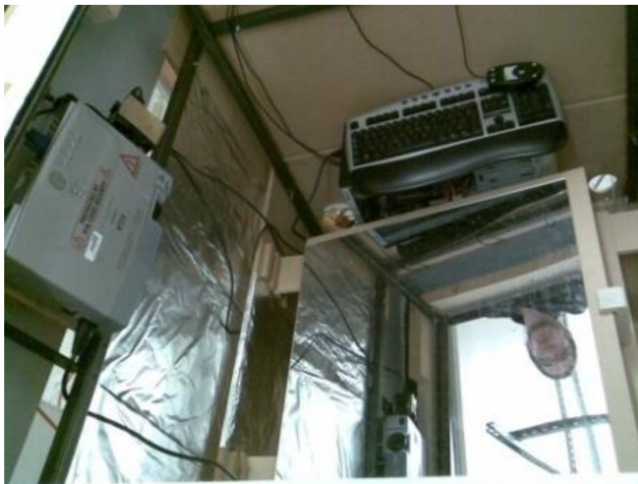
Figure 26: Inside the table, now with the projector mounted. The mirror is hinged and raised at an angle. Note the aluminum foil on the inside of one side panel. This picture was taken during our investigation into reflective/diffusive finishes.
