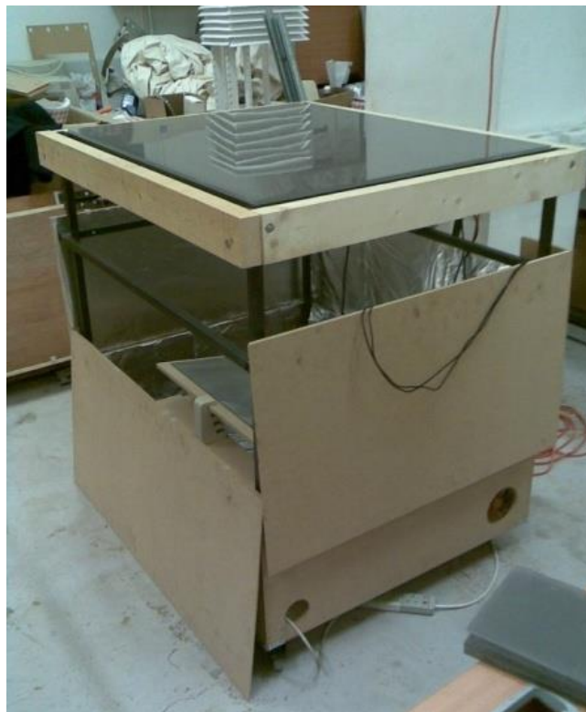
Figure 28: The table before painting. Notice the wooden support beams screwed to the metal frame. The table's lid needs to take the weight of four people leaning on it.
