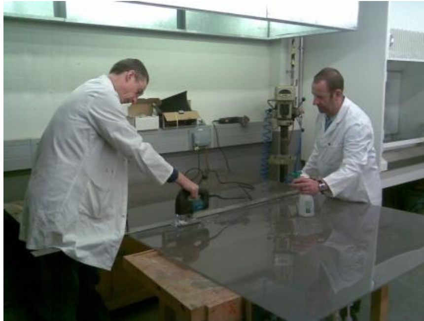
Figure 21: This polycarbonate sheet was originally a spare wall from an old CAVE system at UCL. For this reason, it is an excellent projection surface and happens to be suitably diffuse on one side.
