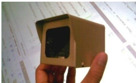
Figure 11: Infrared LED illuminator. As this is a 'night-vision' CCTV illuminator, black tape was placed over the unit's light sensor to force it to turn on.
