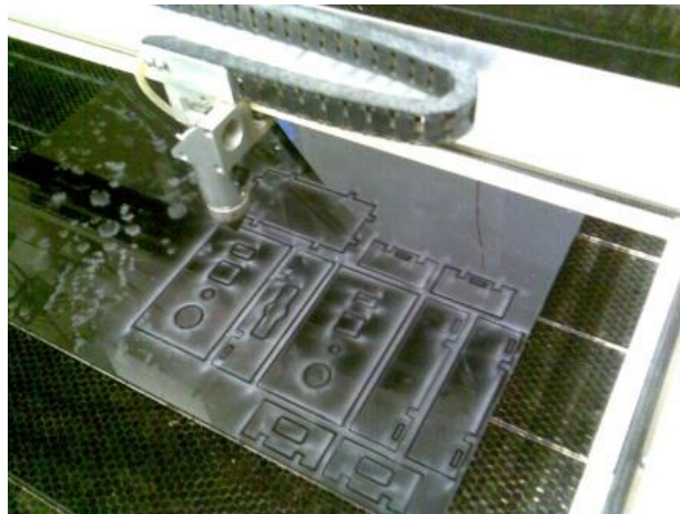
Figure 32: A small switch box was laser cut and assembled. It is situated between the Perspex and sides in a discrete location. The buttons face the floor so that people cannot accidentally reset the system with their knees.
