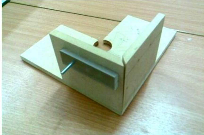
Figure 29: Mock ups are fundamental for deciding the right strategy for a detail. In this case, the lid of the table was mocked up to help decide how more expensive finishes would be applied.
