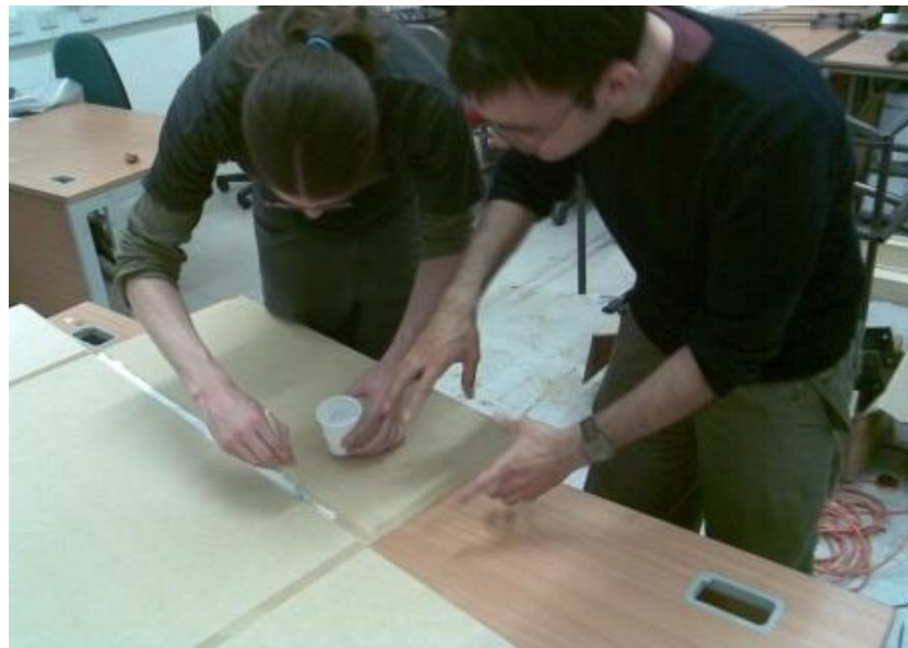
Figure 24: The table base was constructed from MDF. It was first glued and then later strengthened with corner brackets.
