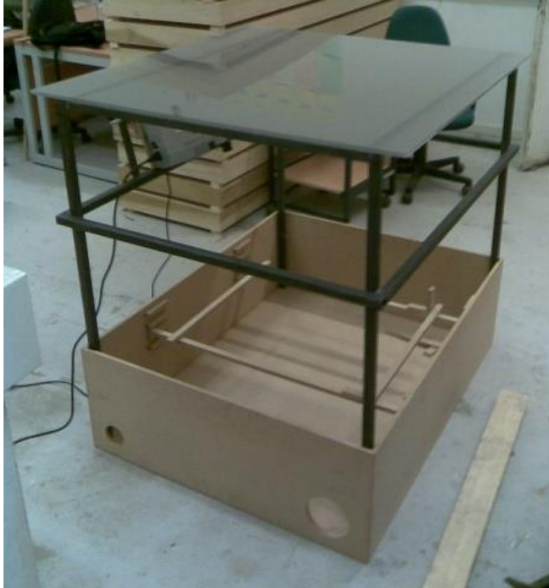
Figure 25: Completed base, steel structure, and (not final sized) polycarbonate surface.
