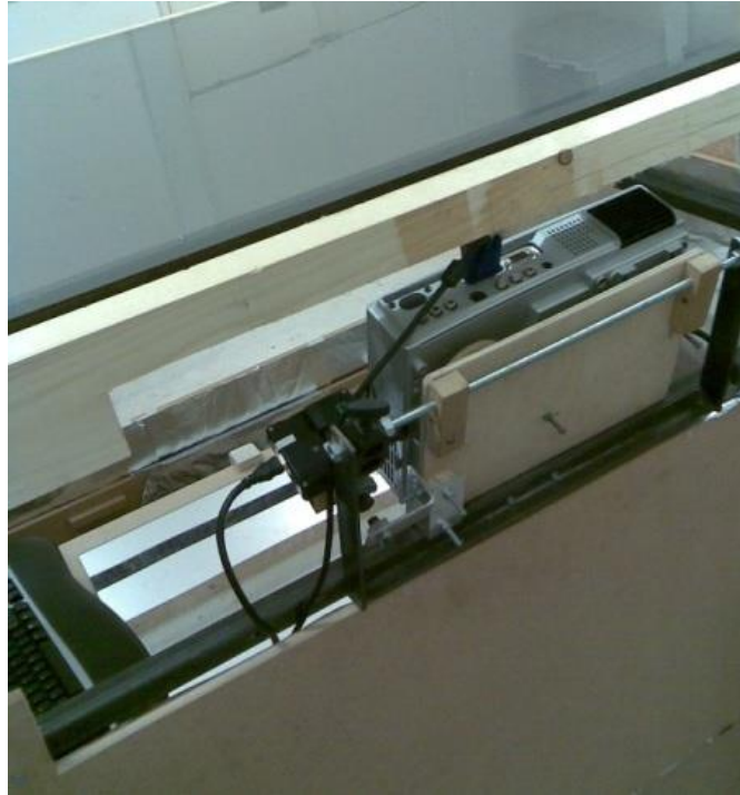
Figure 27: The projector in its metal frame sits inside the table and is invisible from the outside once covered with the lid. The projector's metal frame was designed and constructed to be adjustable and accommodate a variety of models and specifications.
