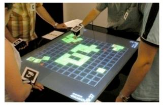
Figure 6. Interacting with multi-touch tabletop through glovebased marker tracking.
