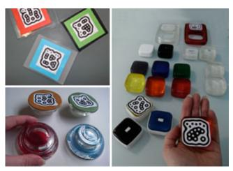
Figure 5. Iterative development of tangible artefacts with printed fiducials. Perspex and paper (top left); glass and leather (bottom left); crystal resin (right).
